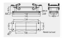
**Bulkhead Mounted Housings** (Assemble the inserts in reverse direction)
